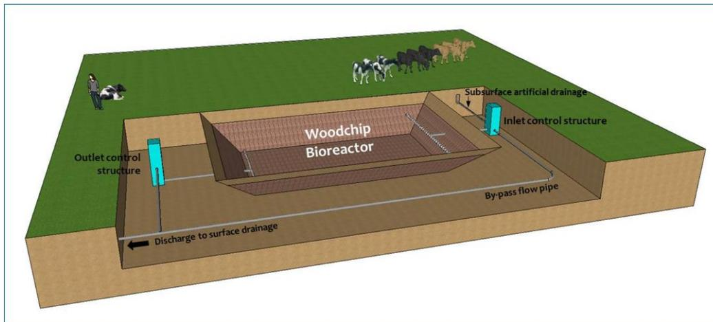
Schematic of the woodchip denitrifying bioreactor
